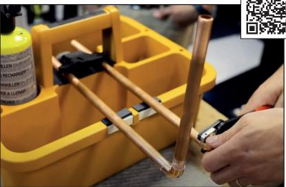
**The Monument Sweatbox**® allows engineers to solder or sweat a new joint up to **22mm** diameter, on site, in a domestic property without having to cobble together some kind of makeshift holding device.
