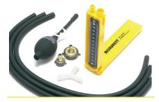
The Monument Drain Test Kit. Use the kit to carry out an air test to 100mm wg pressure (10mb) on drain. Includes U Gauge, bellows pump, 1/2in. BSP & 1in. BSP nipple caps, T piece; 3 x 600mm lengths of rubber hose. Supplied in tube.
