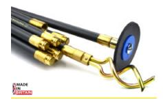
The Monument DIY Drain Rod Set. Rotate 19mm rods clockwise only. Set includes 100mm (4in.) rubber plunger, 100mm (4in.) brush & 50mm (2in.) double worm screw. 10 rods. Rod length 9m (30ff). Universal Joint. Diameter 19mm (3/4in.)
