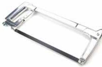
The ENT1921 300mm (12inch) Hacksaw has a die-cast aluminium handle and square section tubular steel frame, which combine to give a lightweight hacksaw with great tensile strength. Adjusts to give 45° angle for flush cutting.
